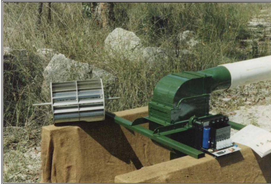
Figure 6 runner, housing and AERL Hydromax controller
